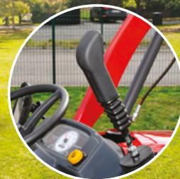
Joystick commande hydraulique
